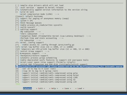
This increases the size of the kernel so take that into account as the kernel is read into DDR by U-Boot.
