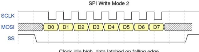
Clock idle high, data latched on falling edge
