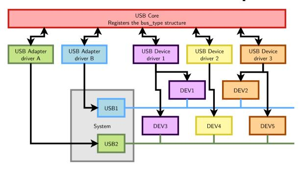
A single driver for compatible devices, though connected to buses with different controllers.
