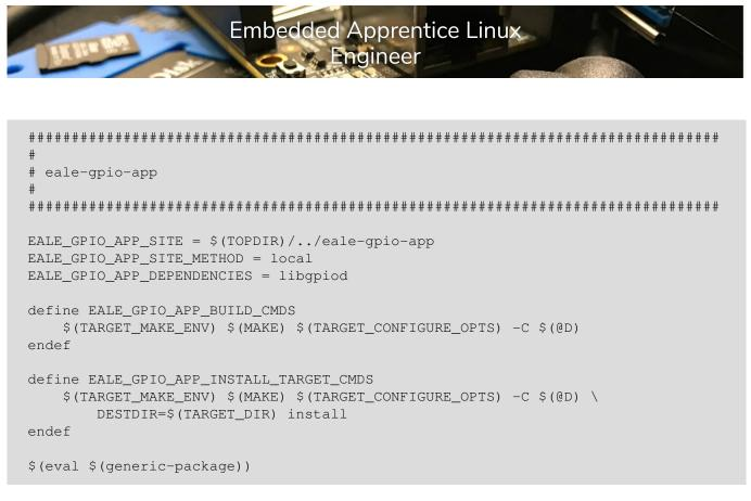
Make sure that the lines inside EALE\_GPIO\_APP\_BUILD\_CMDS and EALE\_GPIO\_APP\_INSTALL\_ TARGET\_CMDS are prefixed with one tab.
